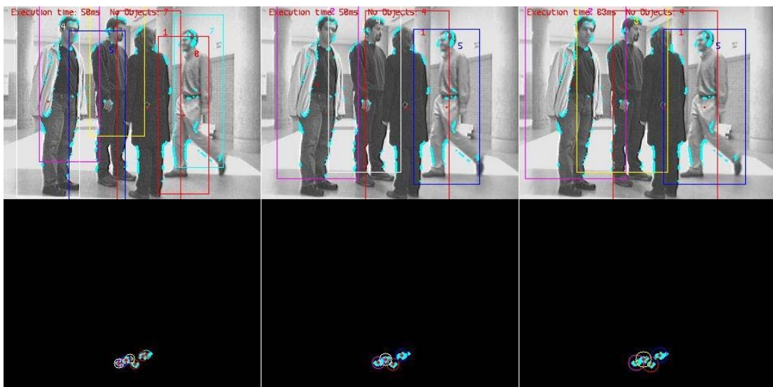
Figure 6.9: Result of a test with three different cylinder radiuses 600 mm to the left, 850mm in the middle and 1000 mm on the right.
