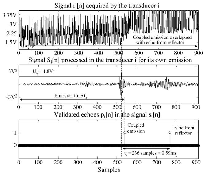
Fig. 13. Real data from a reflector placed at 10 cm (inside the blind zone) for a 32-bit codified ultrasonic emission.
