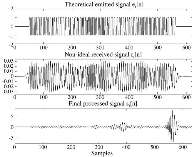
Fig. 9. Example of a 32-bit encoded emission for a whole reception.
