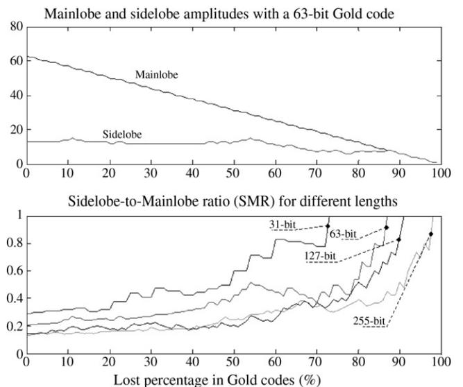
Fig. 2. Behaviour of Gold codes when losing a percentage of the sequence.
