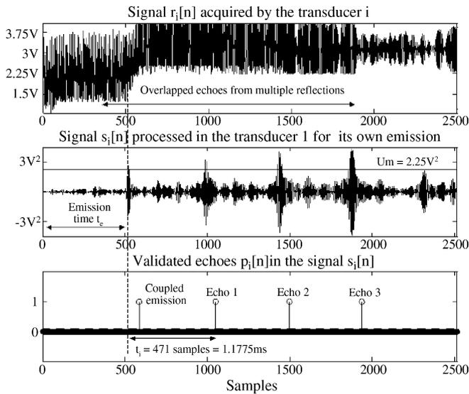
Fig. 12. Real data from a reflector placed at 20 cm (inside the blind zone) for a 32-bit codified ultrasonic emission.
