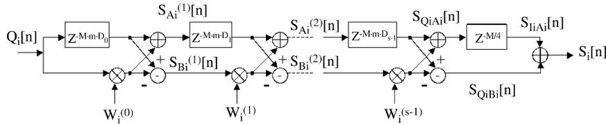
Fig. 7. Modified block diagram of the Efficient Golay Correlator (EGC).
