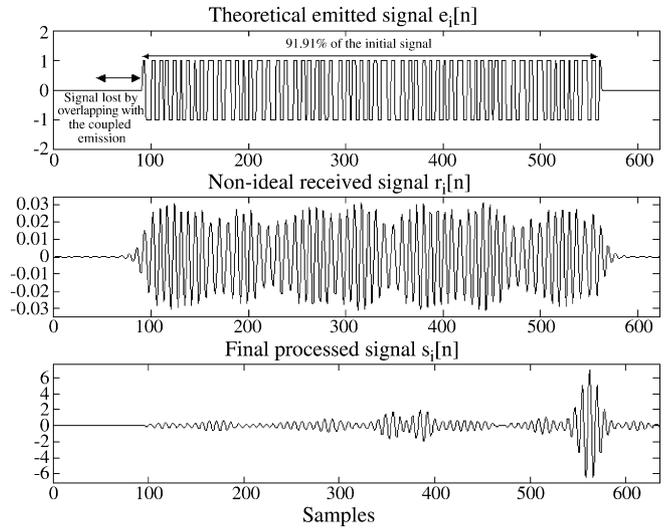
Fig. 11. Example of a 32-bit encoded emission losing the 8.09% initial echo; equivalent to a reflector placed at 10 cm.
