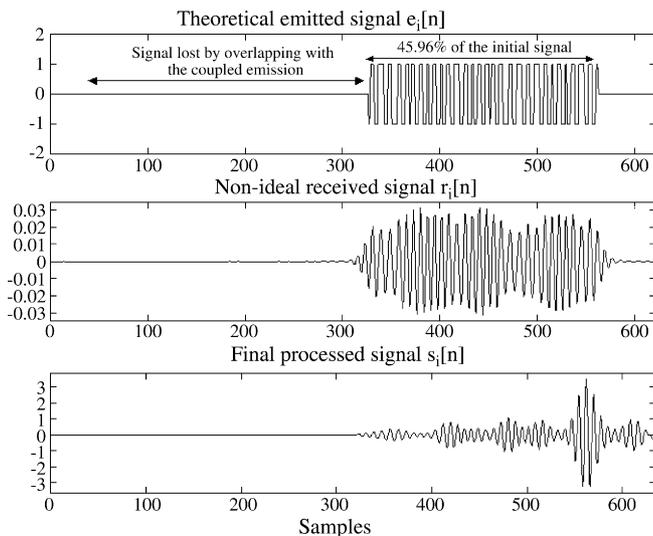
Fig. 10. Example of a 32-bit encoded emission losing the 54.04% initial echo; equivalent to a reflector placed at 20 cm.
