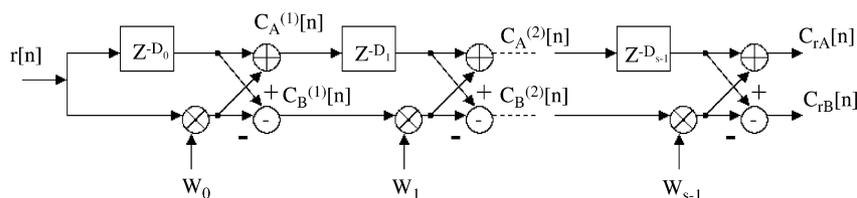
Fig. 6. Block diagram of the Efficient Golay Correlator (EGC).
