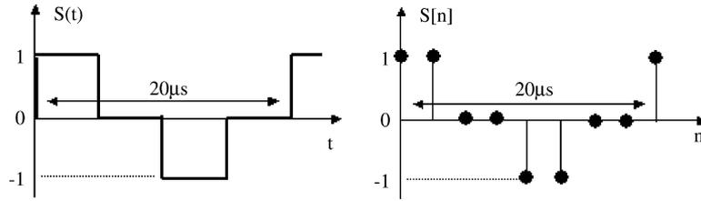
Fig. 5. Symbol  $S[n]$  used in the QPSK modulation.
