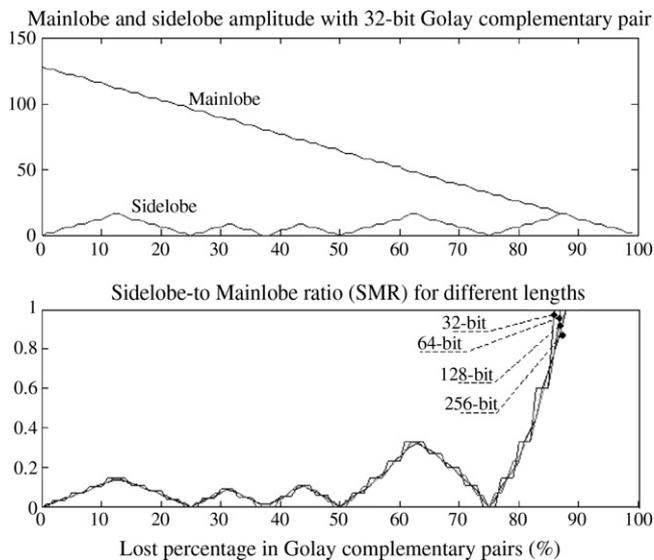
Fig. 4. Behaviour of Golay complementary pairs when losing a percentage of the sequence.
