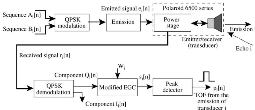
Fig. 8. Block diagram of the processing associated to a transducer  $i$ .
