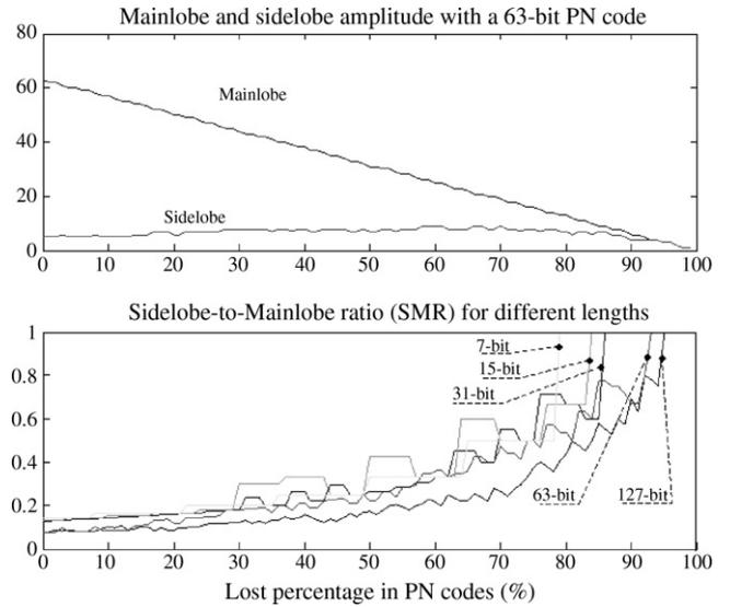
Fig. 1. Behaviour of PN sequences when losing a percentage of the sequence.
