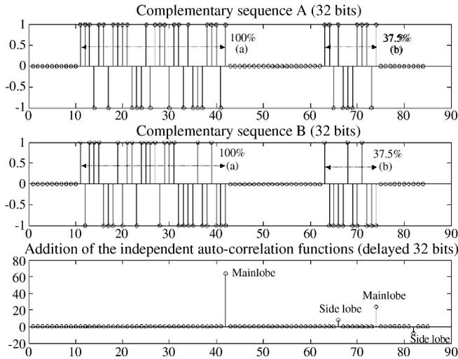
Fig. 3. Example of an auto-correlation function for a 32-bit Golay complementary pair. Two cases are described: (a) the whole sequences are received; (b) the beginning of the sequences is lost (only 37.5% is considered).
