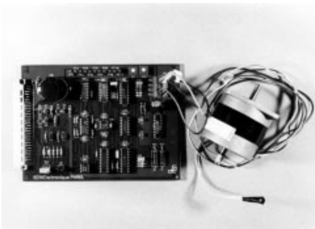
Fig. 9. Photograph of the driving board for stepper motors.
