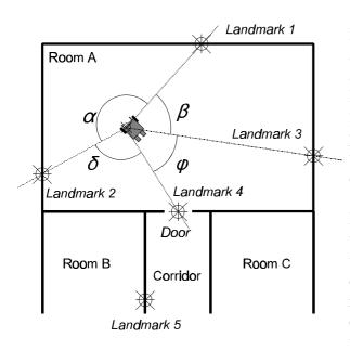
Figure 3.- Landmark absolute positioning
